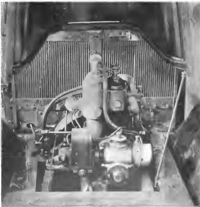
TWO-CYLINDER RENAULT ENGINE OF 8-HORSEPOWER.
